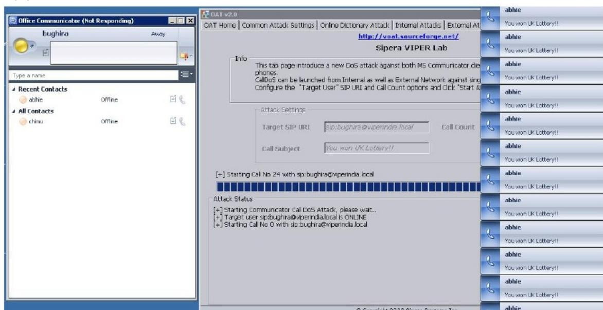
OCS and Lync do not terminate idle calls and does not keep track of ongoing call sessions for particular users, causing this attack to be extremely effective.
