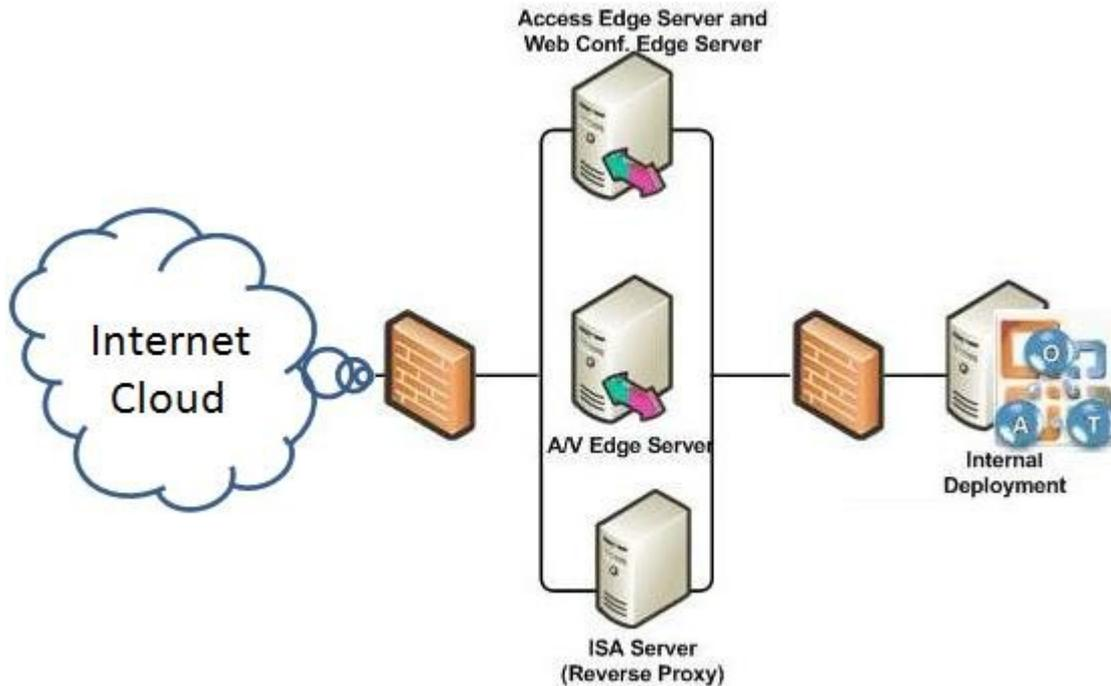
External Network is a deployment scenario where OCS users have to connect through the Edge server. This connection is usually over TLS and users do not have access to the domain controller unless they are connected via VPN.
